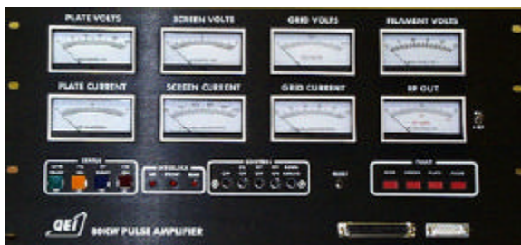
Metering and Control Panel
